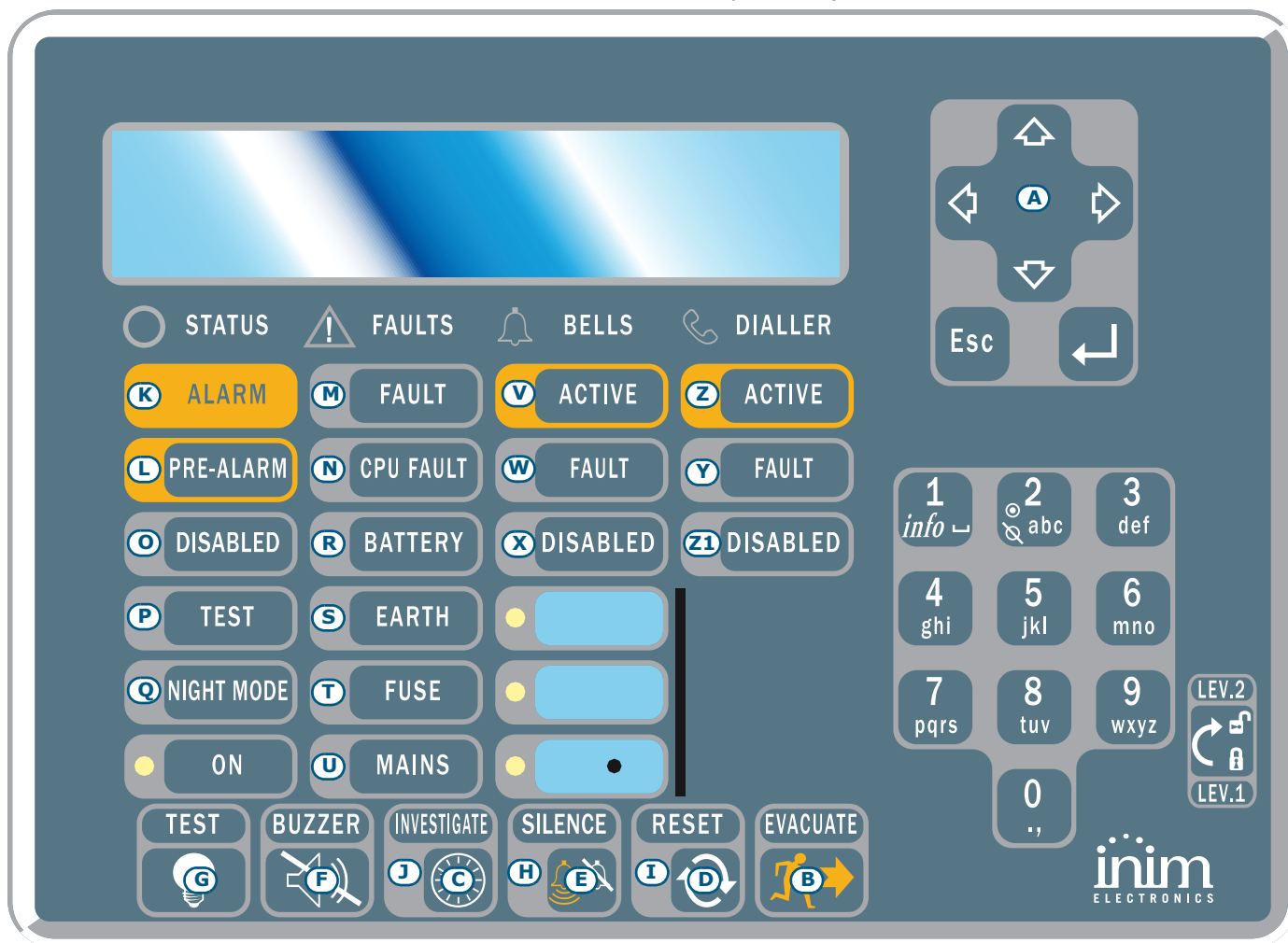
Figure 9 - Front view of the repeater panel
